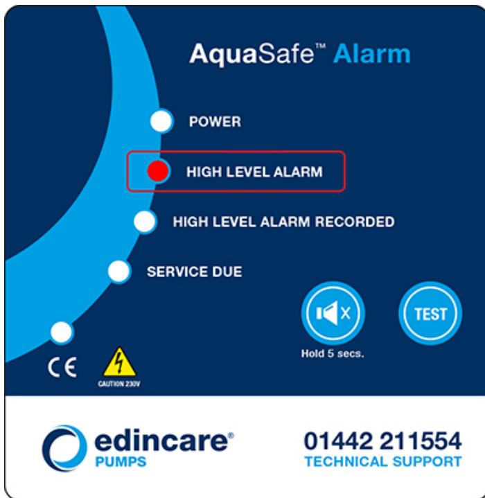
Fig.12 The high level alarm indicator
